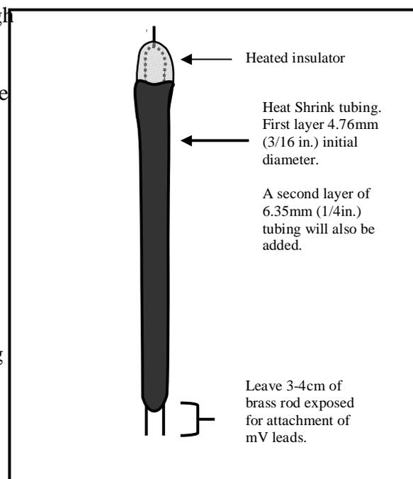
copper wire. You may apply a third layer of tubing at the point where the brass rod and copper wire meet for added protection and stability.
