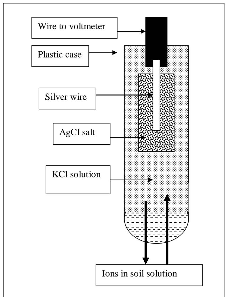
The Ag/AgCl electrode consists of a Ag metal wire and a AgCl salt. The basic reaction is:
