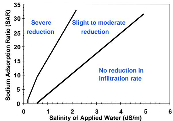
Figure 3. Interaction of total salinity as EC with the sodium adsorption ratio of applied water for causing potential infiltration problems. (Ayers, R.S. and D.W. Westcott. 1985. Water quality for agriculture. United Nations FAO Irrig & Drainage Paper No. 29.)
