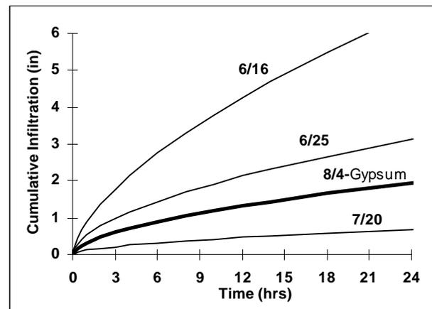
Figure 1. Cumulative depth of infiltration for Wasco sandy loam over the season for the same furrows in furrow irrigated cotton at the Shafter Field Station (Shafter, CA 1995) with low salinity canal water (0.02 dS/m).
