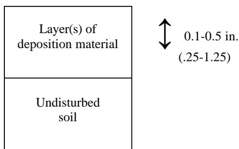
Figure 3. Depositional soil crusting
