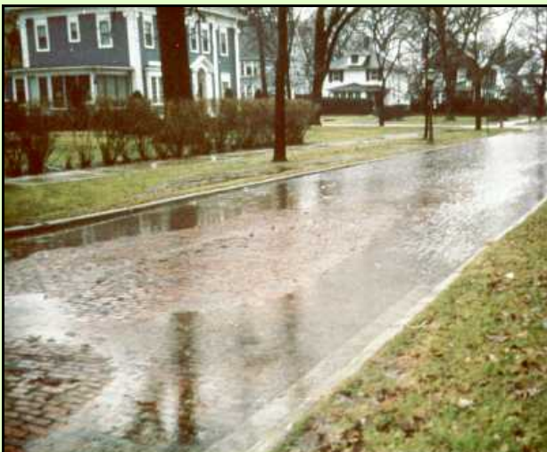
Figure 1. Runoff temporarily stored on a street surface.
