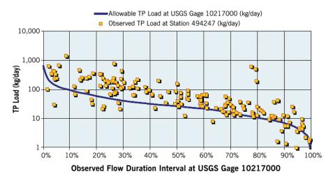
Figure 7. Load duration curve for the Sevier River near Gunnison, UT, January 1977 through September 2002. Blue line represents allowable total P load calculated as the product of each observed flow duration interval and the target total P concentration of 0.05 mg/L. Yellow points represent observed total P loads at the same flow duration intervals.
