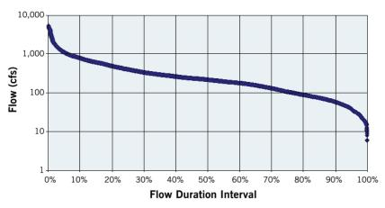
Figure 6. Flow duration curve for the Sevier River near Gunnison, UT, covering the period January 1977 through September 2002.
