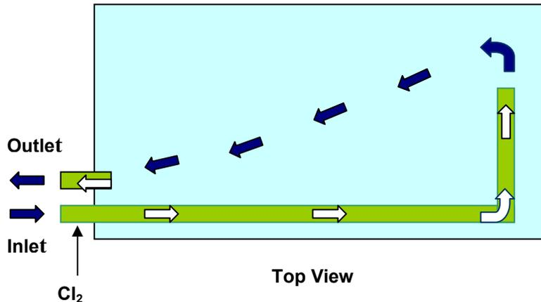
When determining the **time of contact** of the chlorine with the water in the chlorine contact chamber, we therefore must account for **short-circuiting**.
