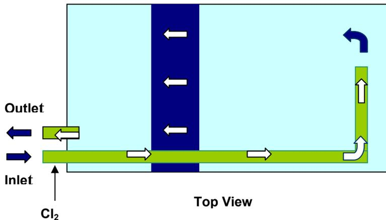
If all the water travelled through the reservoir at an average velocity, the water would travel into the reservoir through the inlet pipe and across the reservoir as a single unit, at an average velocity. There would be **No Mixing** and **No Short-Circuiting**.
