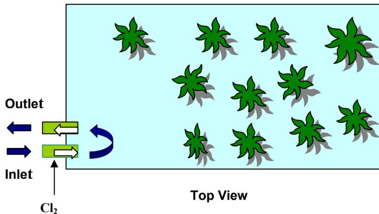
As an absolute minimum, the distance from the inlet to the outlet pipes should be maximized as illustrated in Figure 9. Although short circuiting is still significant, this configuration is a big improvement over the adjacent inlet and outlet pipe scenario.
