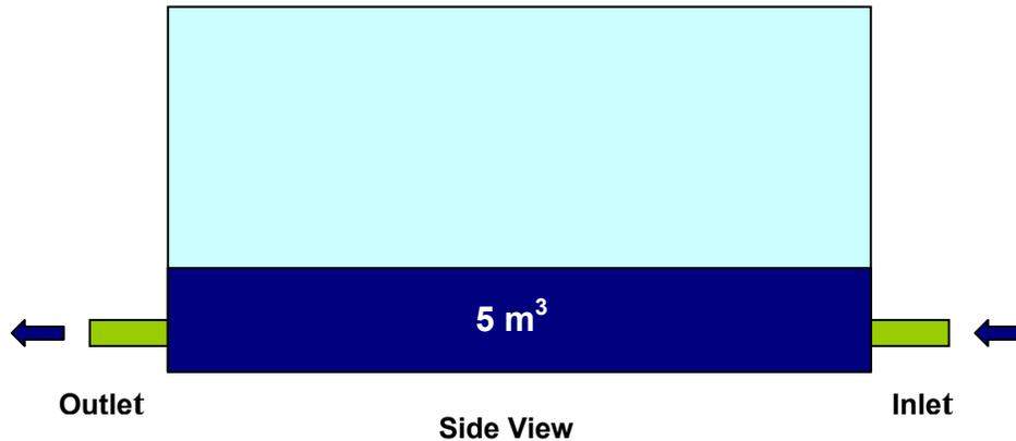
Increasing the minimum volume of water in storage to  $15 \text{ m}^3$ , increases the minimum contact time three fold. We can do this by resetting our flyght bulbs so that the distribution pumps kick out when the water in storage drops to  $15 \text{ m}^3$ , or we can install a weir that holds back at least  $15 \text{ m}^3$  at all times as illustrated in Figure 7.
