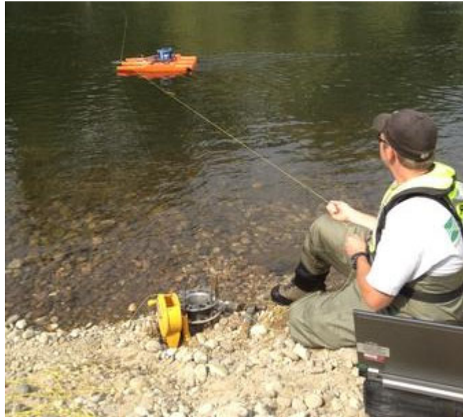
U.S. Geological Survey hydrologic technicians use an acoustic Doppler current profiler to measure streamflow on the Boise River in Boise's Veterans Memorial Park as part of a study of phosphorus mass balance.
