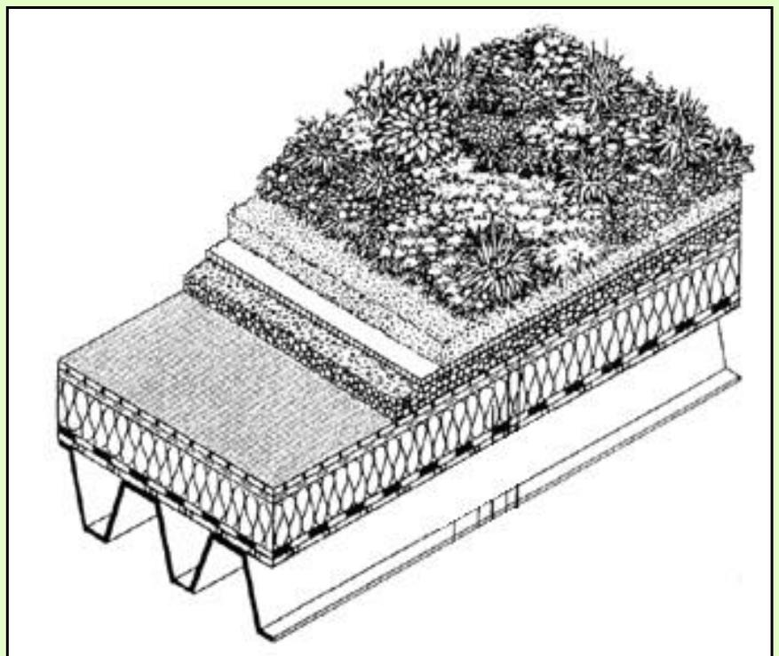
Figure 2. Components of the vegetated roof cover.
